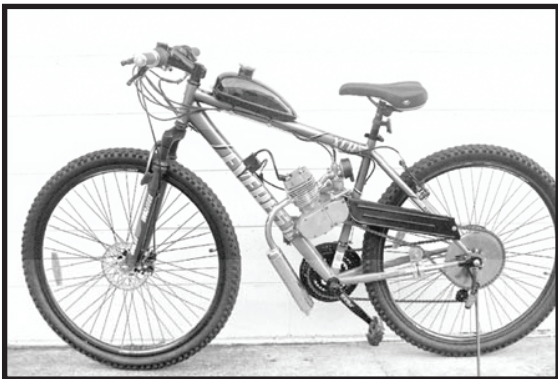
The over-sized "Down Tube" & large number of Spokes makes this "Everest" install a challenge
