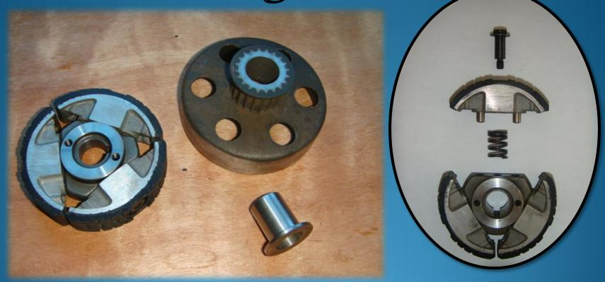
3 shoe pads held by spring tension activated by centrifugal force:
