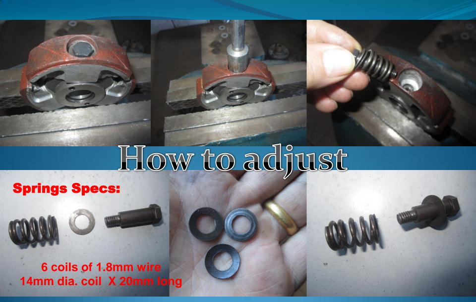
Use a thin wall socket to remove 3 should bolts.
